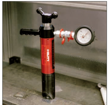
Pull-out test of an ENP fastening with a HAT28 tester and X-ENP adapter
