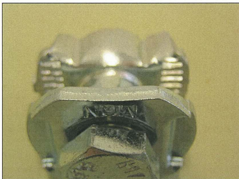
Pic. 20: Screw with toothed lock washer
